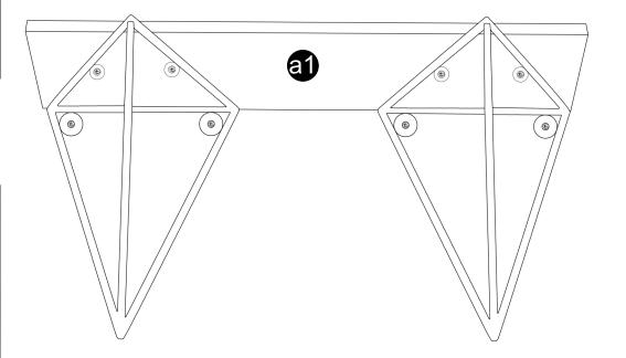
Hang the rack you prepared into the wall dowels by screwing.
