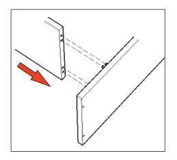
Attach parts 8 to parts 3-4 and 5
