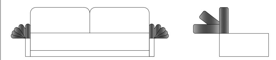
Backrest mechanisms working independently from each other and each offering 3-steps of movement.
